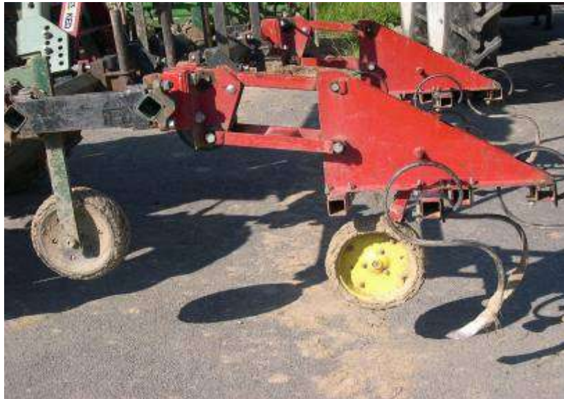
Rear set up with S tines in wheel tracks and side knives on bed (retracted in picture)
