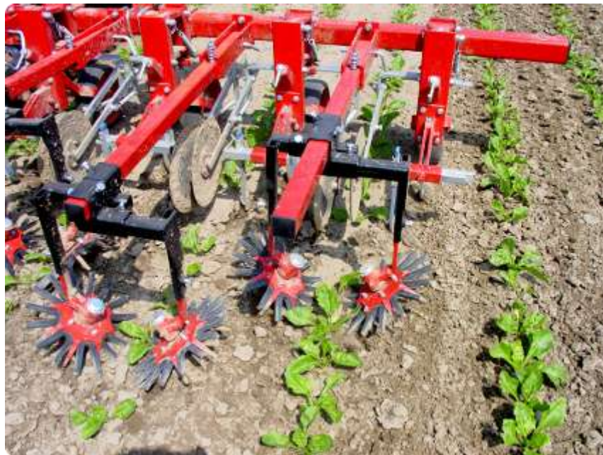
Front mounted Steketee fingerweeder for 2 and 3 row cultivation
