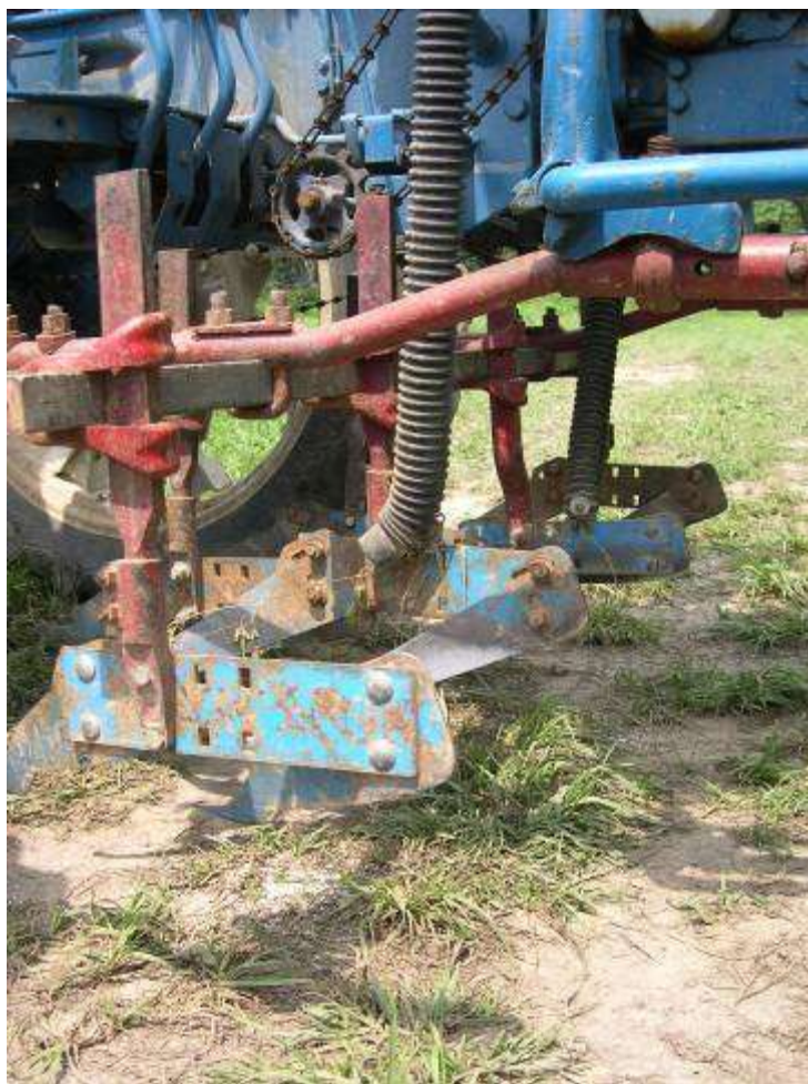
Belly mounted Bezzers springhoes (3 row)
