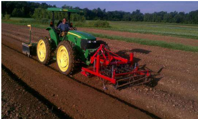
Front and Rear view of combo seedbed maker and bedshaper.
