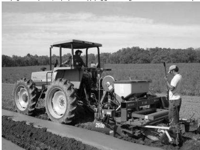
Laying BioTelo plastic, driptape and applying granular organic fertilizer with mulch-layer
