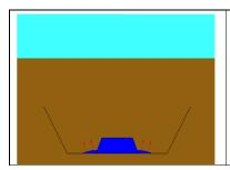
This is resolved in the wicking bed system water by applying water to the bottom of the pond where it is pulled upwards to the roots of the plant by surface tension or wicking action. The water is now not stagnant but continuously moving from the base of the pond upwards to the roots. First in first out.
